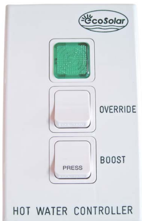
Figure 6: “One Shot” Backup heating controller, allows manual control of the backup heating. The heating is manually turned on and will be automatically turned off, ensuring the element is not left on unintentionally.
