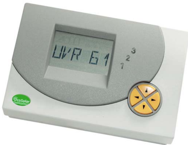
Figure 3 Modern solar controller with a variable speed drive giving it the design duty, maximum torque on start up to reduce the potential of seized pumps and reduced flow rates during pumping to reduce mixing within the cylinder.
